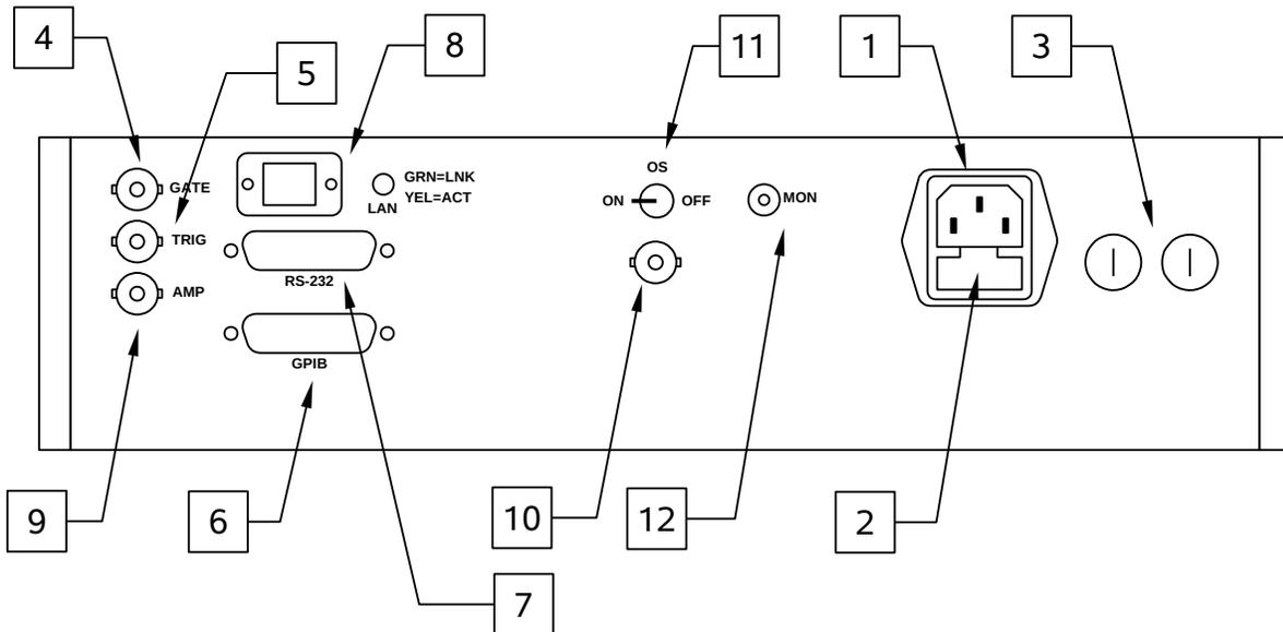
1. AC POWER INPUT. An IEC-320 C14 three-pronged recessed male socket is provided on the back panel for AC power connection to the instrument. One end of the detachable power cord that is supplied with the instrument plugs into this socket.
