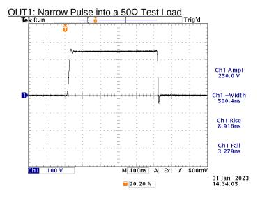
Output of "OUT1" connector, terminated into an external 50 Ohm test load. Viewed with TDS3052 scope. 100V/div, 100 ns/div. 10 Hz.
