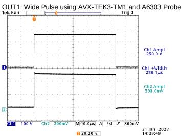
Top: +250V voltage waveform (measured at clamping cable). Bottom: Output of A6303 probe, viewed with TDS3052 scope. The A6303 probe is clamped to the shorting cable.
