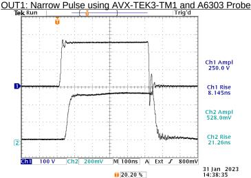
Top: +250V voltage waveform (measured at clamping cable). Bottom: Output of A6303 probe, viewed with TDS3052 scope. The A6303 probe is clamped to the shorting cable.
