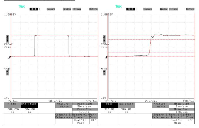
20 V/div (200 mV/div x 40 dB), 50 ns/div. "OUT2" into a sampling oscilloscope.
