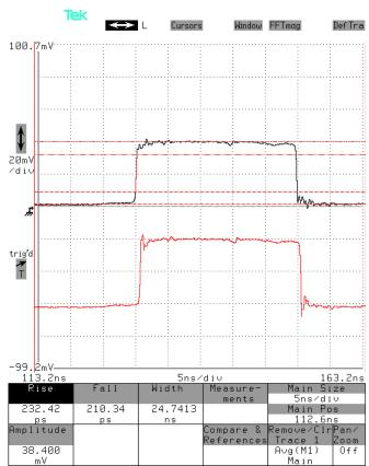
Top: Voltage measured across the resistor in response to a +4.8V pulse applied from an Avtech AV-1030-C pulse generator. It should be approximately (+4.8V / 54.55 $\Omega$ ) × 4.55 $\Omega$  = 400 mV, which agrees with the observed waveform. 200 mV/div (= 20 mV/div × 20 dB), 5 ns/div.
