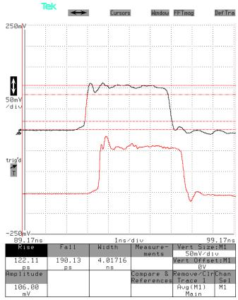
Top waveform: Voltage across the parallel combination of the 4.5  $\Omega$  effective resistance. It should be approximately (+13V / 54.5 $\Omega$ ) × 4.5 $\Omega$  = +1.07V in amplitude, which agrees approximately with the observed waveform.
