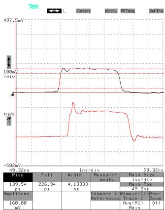
Top waveform: Voltage across the parallel combination of the 4.5  $\Omega$  effective resistance. It should be approximately (+20V / 54.5 $\Omega$ ) × 4.5 $\Omega$  = +1.65V in amplitude, which agrees approximately with the observed waveform.
