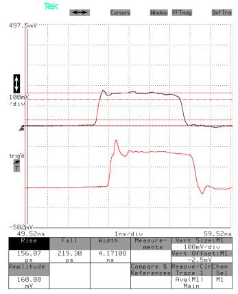
Top waveform: Voltage across the parallel combination of the 4.5  $\Omega$  effective resistance. It should be approximately  $(+20V / 54.5\Omega) \times 4.5\Omega =$ +1.65V in amplitude, which agrees approximately with the observed waveform.
