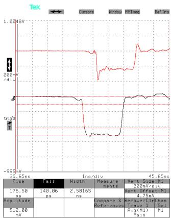
Bottom: "MI" output. 1V/div ( $100 \text{ mV/div} \times 20 \text{ dB}$ ). This shows that the pulse amplitude after the inverting transformer is  $-1.2V \times 11 = -13.2V$ , approximately. (There is  $\sim 12\%$  loss in the transformer).
