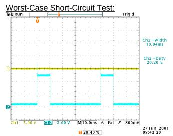
Top: OUT, 4.5A amplitude with 0.5A offset, into  $0\Omega$  10ms PW, 20 Hz PRF, 5V/div, 10 ms/div Bot: Monitor output into  $10k\Omega$  load, 2V/div, 10 ms/div
