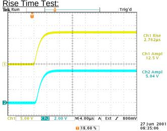
Top: OUT, 5A into  $2.5\Omega$  load, zero offset, 10ms PW, 20 Hz PRF, 5V/div, 4 us/div Bot: Monitor output into  $10k\Omega$  load, 2V/div, 4 us/div
