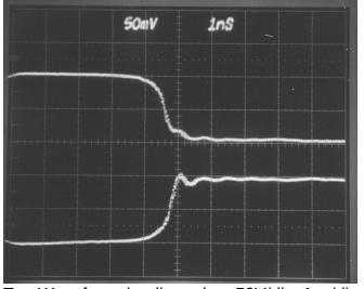
Top Waveform: leading edge, 50V/div, 1ns/div Bottom Waveform: trailing edge, 50V/div, 1ns/div
