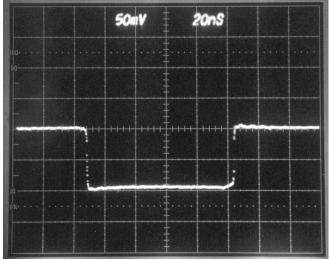
50V/div, 20ns/div. First pulse in 12 pulse burst, with 350 ns spacing , 1 kHz burst rate, -100V amplitude.
