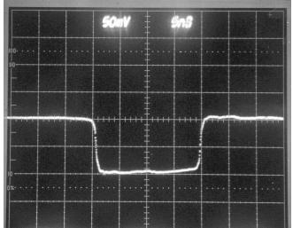
50V/div, 5ns/div. First pulse in 12 pulse burst, with 350 ns spacing , 1 kHz burst rate, -100V amplitude.
