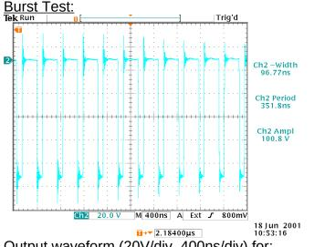
Output waveform (20V/div, 400ns/div) for: Burst Rate=1 kHz, PW=100ns, AMPL=-100V, 12 pulses in burst, with 350 ns spacing. The overshoot and ringing are artifacts of the bandwidth-limited (500 MHz) reattime oscilloscope.
