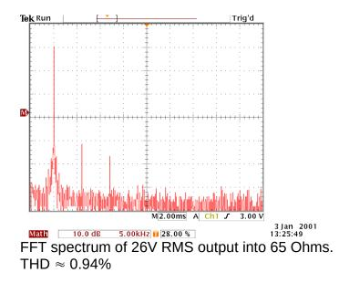
a) Output Signal Amplitude: 26 V<sub>RMS</sub>
