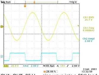
CH1: OUT, 26  $V_{RMS}$  sine wave into a 65 $\Omega$  load CH2: SYNC output, into 50 Ohms
