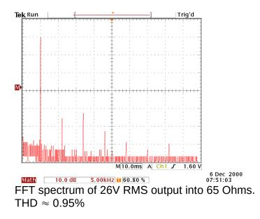
a) Output Signal Amplitude: 26 V<sub>RMS</sub>
