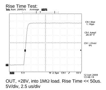
a) Output Signal Amplitude: 0 to +28V
