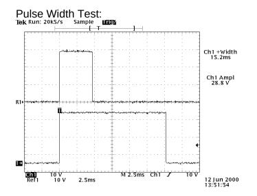
Top: OUT, +28V, 5 ms wide, into  $1M\Omega$  load. Bottom: OUT, +28V, 15 ms wide, into  $1M\Omega$  load. Both: 10 V/div, 2.5 ms/div
