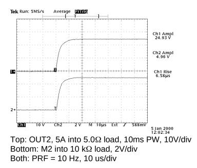
a) Output Signal Amplitude: 0-5A
