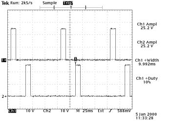
Top: OUT1, 5A into  $5.0\Omega$  load, 10ms PW, 70ms delay Bottom: OUT2, 5A into  $5.0\Omega$  load, 10ms PW Both: 10V/div, 25ms/div, PRF = 10 Hz
