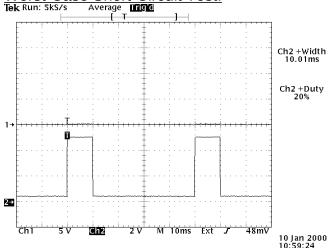
Top: OUT, 4.5A amplitude with 0.5A offset, into  $0\Omega$  10ms PW, 20 Hz PRF, 5V/div, 10 ms/div Bot: Monitor output into  $10k\Omega$  load, 2V/div, 10 ms/div  $I_{AC}$  = 0.97A @ 115  $V_{AC}$  for this test.
