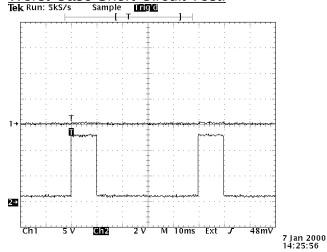
Top: OUT, 4.5A amplitude with 0.5A offset, into  $0\Omega$  10ms PW, 20 Hz PRF, 5V/div, 10 ms/div Bot: Monitor output into  $10k\Omega$  load, 2V/div, 10 ms/div  $I_{AC}$  = 0.97A @ 115  $V_{AC}$  for this test.
