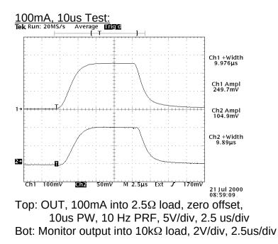
a) Output Signal Amplitude: 0-5A
