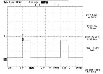
Top: OUT, 4.5A amplitude with 0.5A offset, into  $0\Omega$  10ms PW, 20 Hz PRF, 5V/div, 10 ms/div Bot: Monitor output into  $10k\Omega$  load, 2V/div, 10 ms/div  $I_{AC}$  = 1.0A @ 115  $V_{AC}$  for this test.
