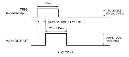
The delay, pulse width, and frequency (when in the internal mode), of the OUT pulse can be varied with front panel controls or via the GPIB or RS-232 computer interfaces.
