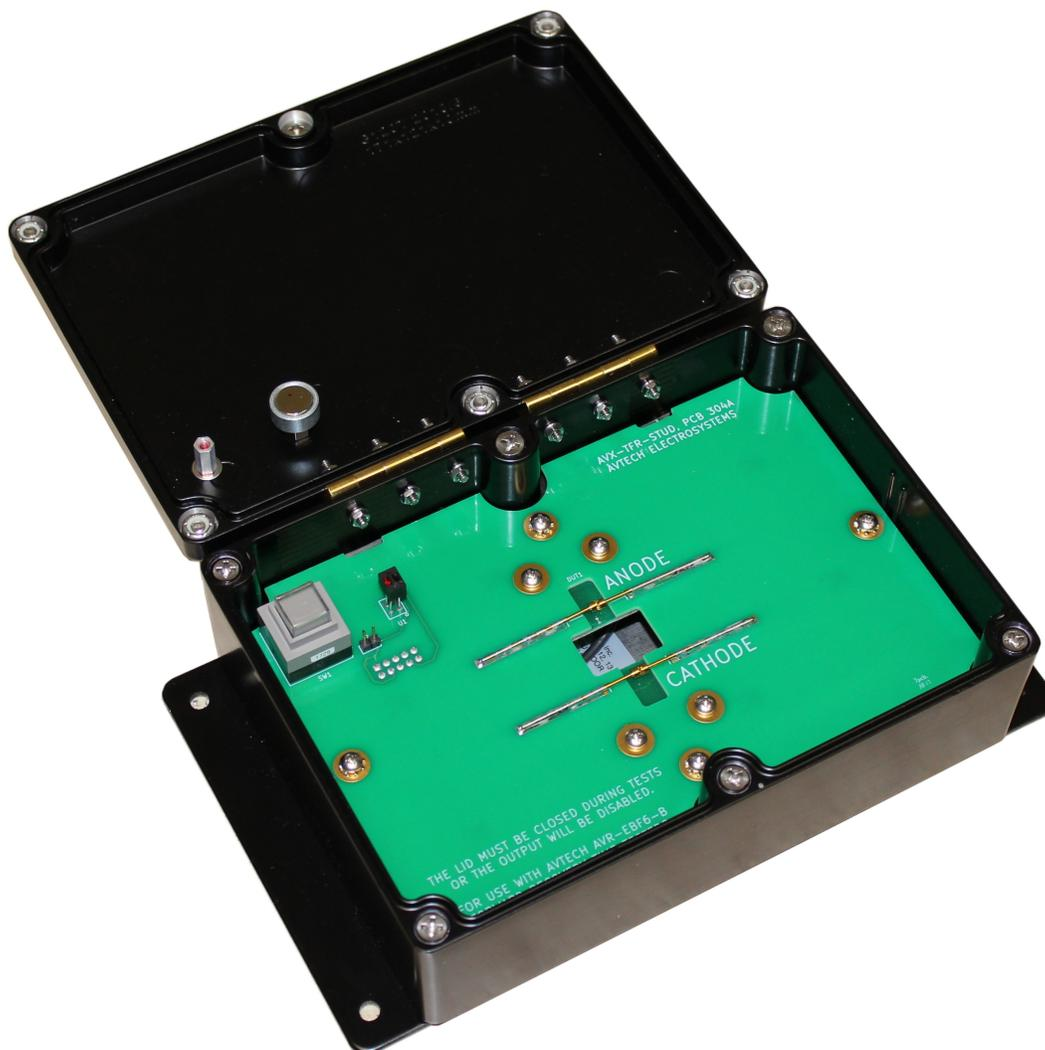
The photo below shows a reverse-polarity DO-4 diode (the Ruttonsha 12FLR60/F05) installed between the four spring-loaded contacts (two for the anode end, and two for the cathode end):
