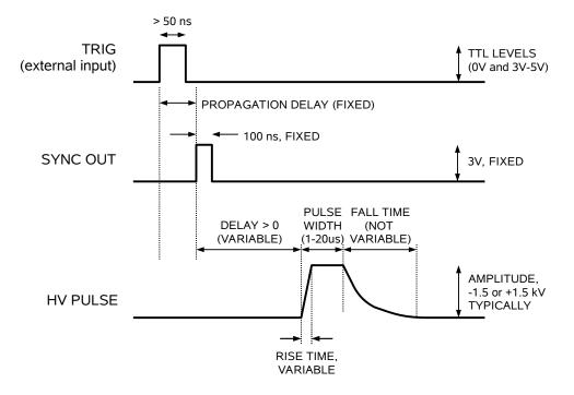
As before, if the delay is negative, the order of the SYNC and OUT pulses is reversed.
