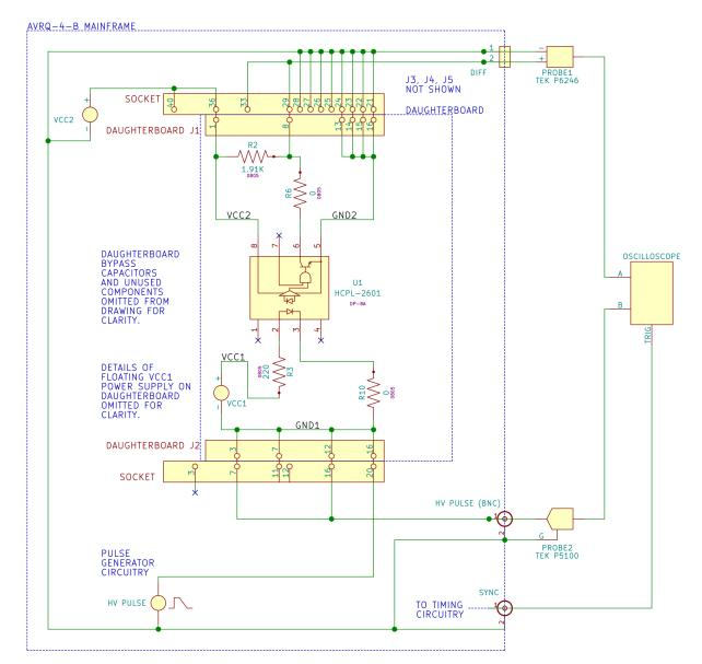
The figure below shows the basic test arrangement for the AVRQ-4-B, with one possible DUT daughterboard configuration, with a high-current input bias on the LED:
