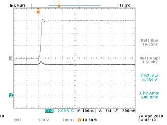
With the high-voltage pulse recorded earlier using the oscilloscope memory function (before being disconnected), no spurious noise is coupled to the logic output signal.
