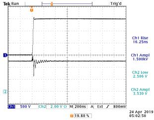
With both the high-voltage pulse and the low-voltage logic output measured simultaneously, inter-channel interference adds significant spurious noise artefacts to the logic signal.
