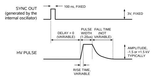
If the delay is negative, the order of the SYNC and OUT pulses is reversed:
