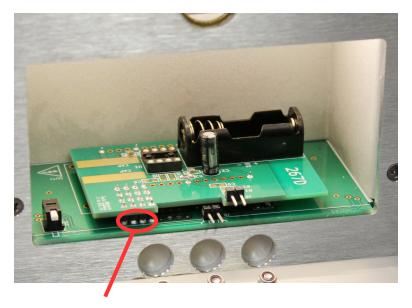
Align the daughterboard with the front-left pin sockets. (Some pin sockets are not used in the AVRQ-4-B.)
