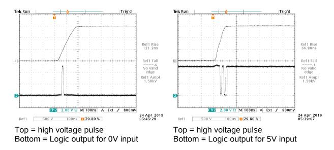
With the daughterboard installed in the socketing in the negative position, and AMP1 set to -1.5 kV and AMP2 set to +5V, these waveforms were obtained:
