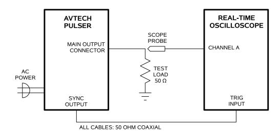
BASIC TEST ARRANGEMENT, WITH A REAL-TIME OSCILLOSCOPE
