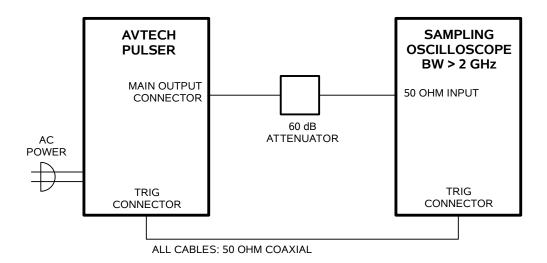
BASIC TEST ARRANGEMENT, WITH A SAMPLING OSCILLOSCOPE
