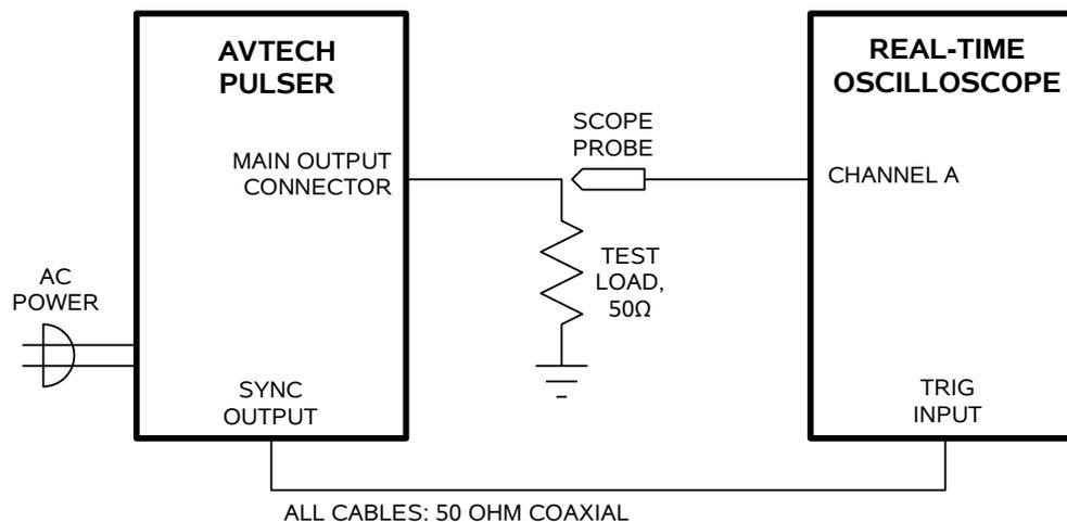
1. Connect a cable from the SYNC OUT connector to the TRIG input of an oscilloscope. Connect a 10 kΩ (or higher) load to the OUT connector and place the scope probe across this load. The load resistor must have a voltage rating of at least 250V. The power dissipated in the resistor is given by
