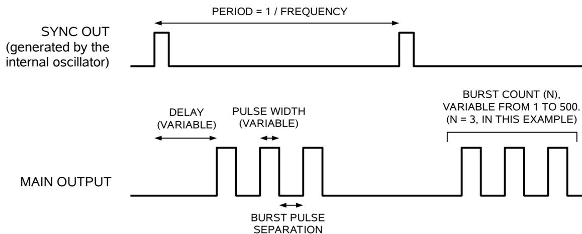
The figure below shows burst mode operation used with external triggering:
