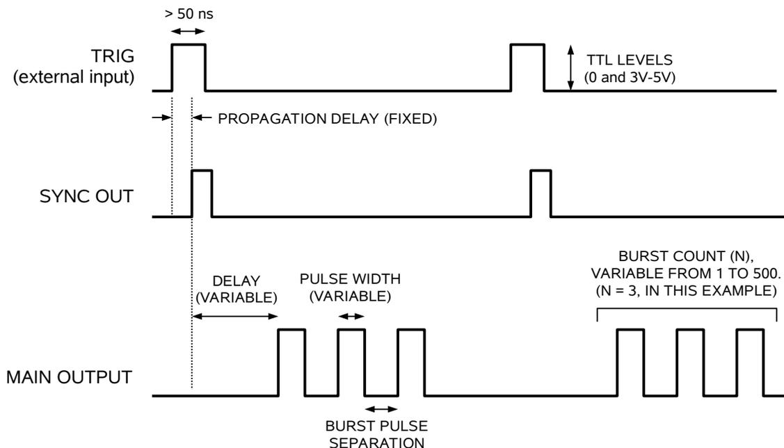
The burst mode may also be used with the front-panel “Single Pulse” pushbutton as a trigger source. (Pressing the pushbutton will actually generate a single burst, rather than a single pulse, in this mode.) Computer commands can also trigger a burst.
