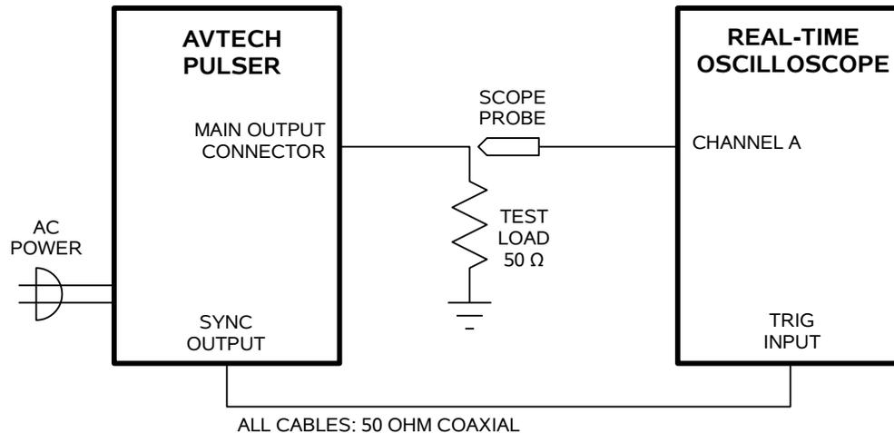
*BASIC TEST ARRANGEMENT, WITH A REAL-TIME OSCILLOSCOPE*
