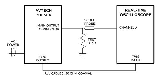
1. Connect a cable from the SYNC OUT connector to the TRIG input of an oscilloscope. Connect a  $50\Omega$  (or higher) load to the OUT connector and place the scope probe across this load. The load resistor <u>must</u> have a voltage rating of at least 700V. The power dissipated in the resistor is given by
