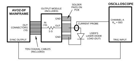
On the output module, the output signal is provided on the larger central pad on the protruding section of circuit board. The two edge pads are grounded. The back side of the board has a solid ground plane.
