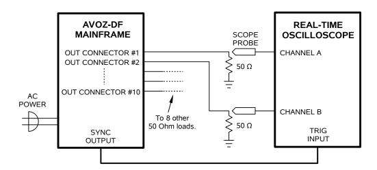
No output should be left unterminated, or reflections may occur on the connected outputs.
