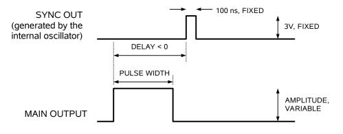
Basic Output Pulses for Delay < 0
