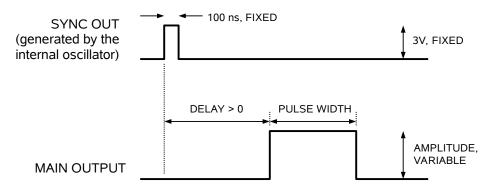
Basic Output Pulses for Delay > 0
