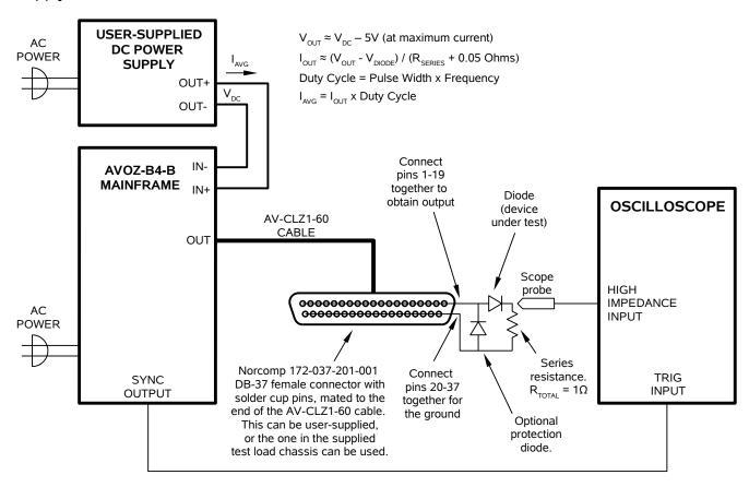
The loads can be connected to the pulse generator using the convenient AV-CLZ1-60 transmission line cable assembly, which has a  $1\Omega$  characteristic impedance ( $Z_0$ ), and is terminated with a DB-37 male connector. A sample low-power connectorized test load is provided for initial testing purposes.
