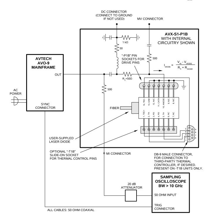
Note: On units with the -OFS1A option,  $R_S$  is reduced from  $50\Omega$  to  $47\Omega$ .
