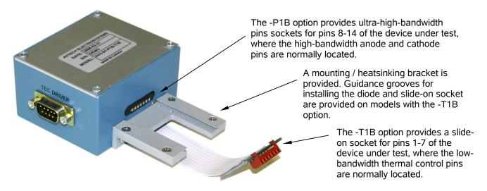
The diode is first installed by sliding pins 8-14 into the "P1B" pin sockets, as shown below:
