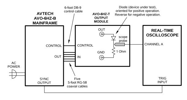
If the AVO-6HZ-B is operated at its maximum duty cycle, the worst-case power dissipation in the output module is  $(110V \times 10A \times 5\%) = 55$  Watts. The internal fan must have sufficient external ventilation to cool the module. The DB-9 control cable must be connected as shown above for the fan to operate.
