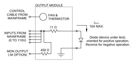
Output Module Functional Equivalent Circuit
