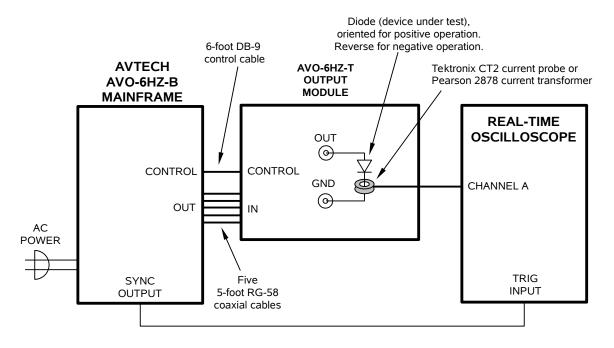
If a Tektronix CT2 current probe or Pearson 2878 current transformer is not available to measure the output current waveform, or the output pulses are too wide, a 1 Ohm resistor may be used to sense the current instead. However, noticeable ringing and
