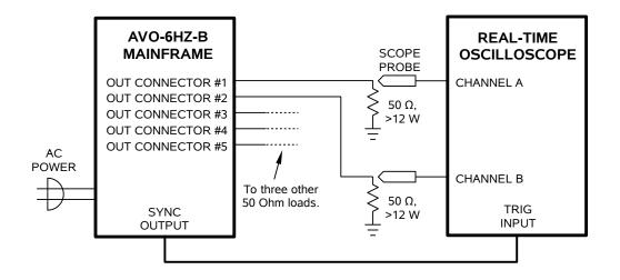
The load resistors must have a voltage rating of at least 110V, and a power rating of at least 15 Watts. They must also be low-inductance, or the waveform will become distorted and exhibit noticeable ringing.
