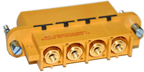
Rear view of the AV-HLZAX adapter. The outer two contact posts are grounded, and the inner two carry the signal. The user may screw into these posts, to attach the user's load. Copper brackets are included (and are normally installed) to jumper the pairs of posts together.
