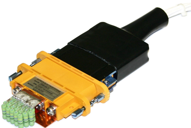
Output end of an AV-HLZ1-100 cable with the AV- HLZAX adapter installed. The supplied copper brackets are installed (one to join the two output posts, and one to join the two ground posts), and some resistors (not supplied) have been soldered to the copper brackets.
