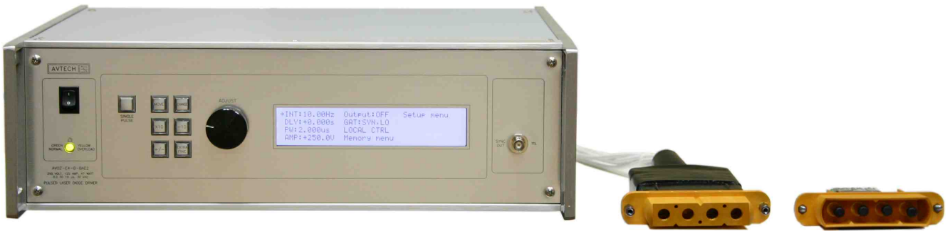
Pulser mainframe (left) with AV-HLZ1-100 output cable (middle) and mating adapter (right)
