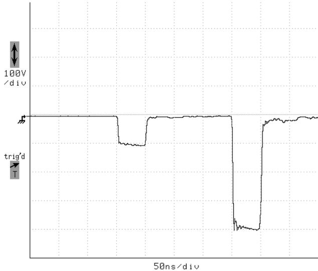
The -DPF option adds the ability to generate pulse doublets, instead of single pulses. The first and second pulses in the doublet have independently variable amplitude and pulse width. Both must have the same polarity. (For dual-polarity models, the polarity setting will affect both pulses in the doublet.)
