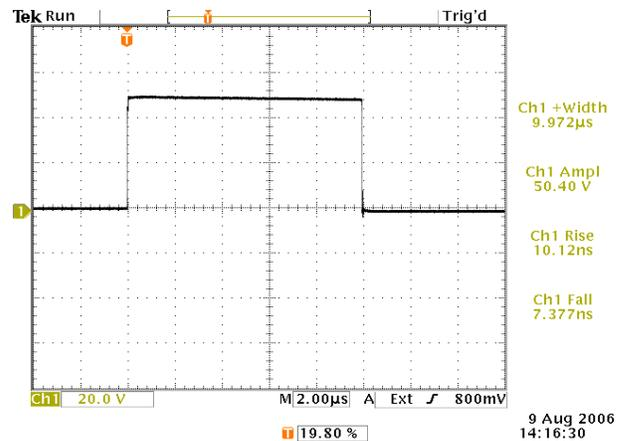
AVX-MRB5 output waveform into 12.5Ω
