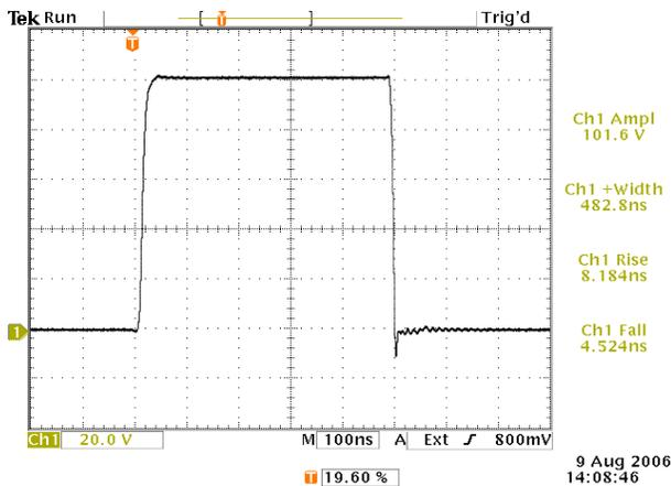
Output of an AV-1010-B into 50 Ohms.
