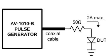
Use a 50 Ohm resistor to match the laser diode to the AV-1010-B. This limits the current to a safe level for the AV-1010-B, and terminates the coaxial cable to minimize ringing.
