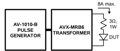
The AVX-MRB6 transformer can be used to quadruple the output current to a maximum of 8 Amps. The load impedance must be reduced by a factor of 16, to 3 Ohms. The maximum pulse width is limited to 10 us.
