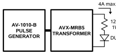
The AVX-MRB5 transformer can be used to double the output current to a maximum of 4 Amps. The load impedance must be reduced by a factor of 4, to 12 Ohms. The maximum pulse width is limited to 10 us.
