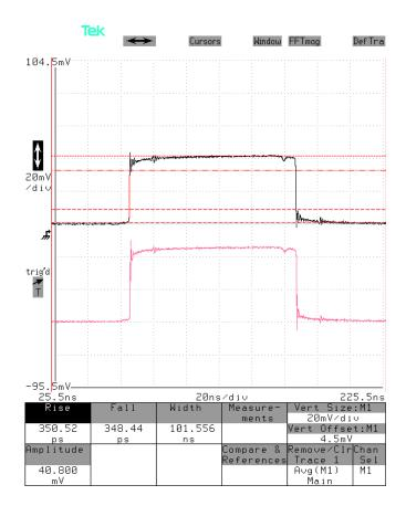
Top: Voltage measured across the resistor in response to a +4.8V pulse applied from an Avtech AV-1030-C pulse generator. It should be approximately  $(+4.8V / 54.6\Omega) \times 4.6\Omega = 404$  mV, which agrees with the observed waveform. 200 mV/div (= 20 mV/div × 20 dB), 20 ns/div.
