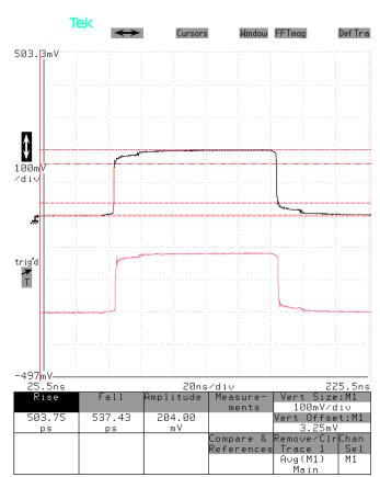
Top: Voltage measured across the resistor in response to a +4V pulse applied from an Avtech AV-1030-B pulse generator. It should be approximately  $(+4V / 50\Omega) \times 25\Omega = +2V$ , which agrees with the observed waveform. 1 V/div (= 100 mV/div × 20 dB), 20 ns/div.
