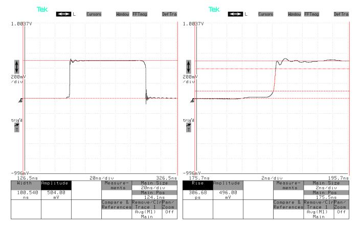
OUT2: 100 ns Pulse into a 50Ω Test Load
