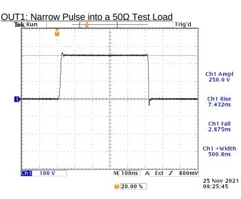
Output of "OUT1" connector, terminated into an external 50 Ohm test load. Viewed with TDS3052 scope. 100V/div, 100 ns/div. 10 Hz.
