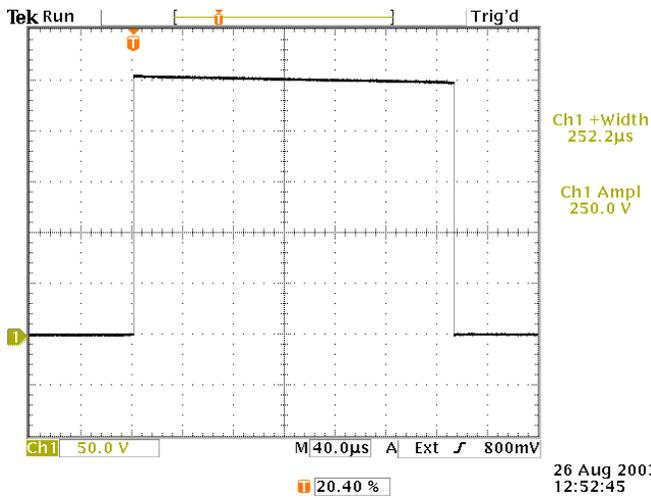
Output of "OUT" connector, terminated into an external 50 Ohm load.
