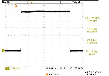
Output of "OUT" connector, terminated into an external 50 Ohm load. Viewed with TDS3052 scope. 50V/div, 400 ns/div.
