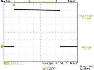
Output of "OUT" connector, terminated into an external 50 Ohm load. Viewed with TDS3052 scope. 50V/div, 40 us/div.
