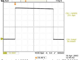
Output of A6303 probe, viewed with TDS3052 scope. The A6303 probe is clamped to the shorting bar.
