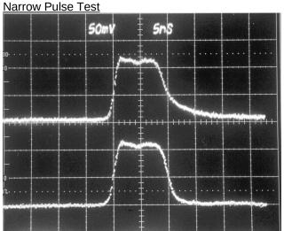
Output waveforms into 60 dB of attenuation. PRF = 1 kHz Top: Narrow pulse using 100-foot cable. 5 ns/div, 50 V/div. Bottom: Narrow pulse using 6-inch cable. 5 ns/div, 50 V/div.
