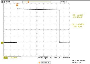
Output of A6303 probe, viewed with TDS3052 scope. The A6303 probe is clamped to the shorting bar.
