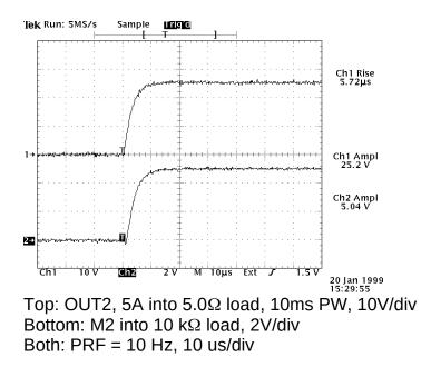
a) Output Signal Amplitude: 0-5A
