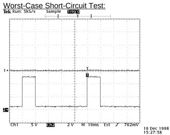
Top: OUT, 4.5A amplitude with 0.5A offset, into  $0\Omega$  10ms PW, 20 Hz PRF, 5V/div, 10 ms/div Bot: Monitor output into  $10k\Omega$  load, 2V/div, 10 ms/div  $I_{AC}$  = 1.03A @ 115  $V_{AC}$  for this test.
