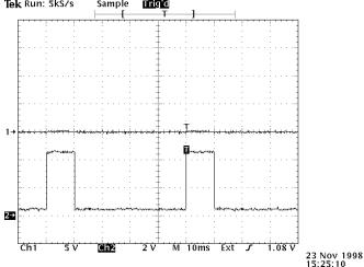
Top: OUT, 4.5A amplitude with 0.5A offset, into  $0\Omega$  10ms PW, 20 Hz PRF, 5V/div, 10 ms/div Bot: Monitor output into  $10k\Omega$  load, 2V/div, 10 ms/div  $I_{AC}$  = 1.03A @ 115  $V_{AC}$  for this test.
