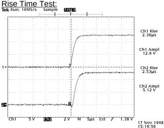
Top: OUT, 5A into  $2.5\Omega$  load, zero offset, 10ms PW, 20 Hz PRF, 5V/div, 5 us/div Bot: Monitor output into  $10k\Omega$  load, 2V/div, 5us/div
